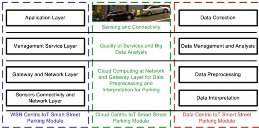
Fig. 5 IoT-based real time smart street parking system architecture
